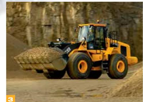
The 467 features wheel speed braking, engine de-rating and intelligent clutch cut-off as standard. A 5-speed transmission with lockup torque converter and automatic differential locking axles complete the efficiency package.
