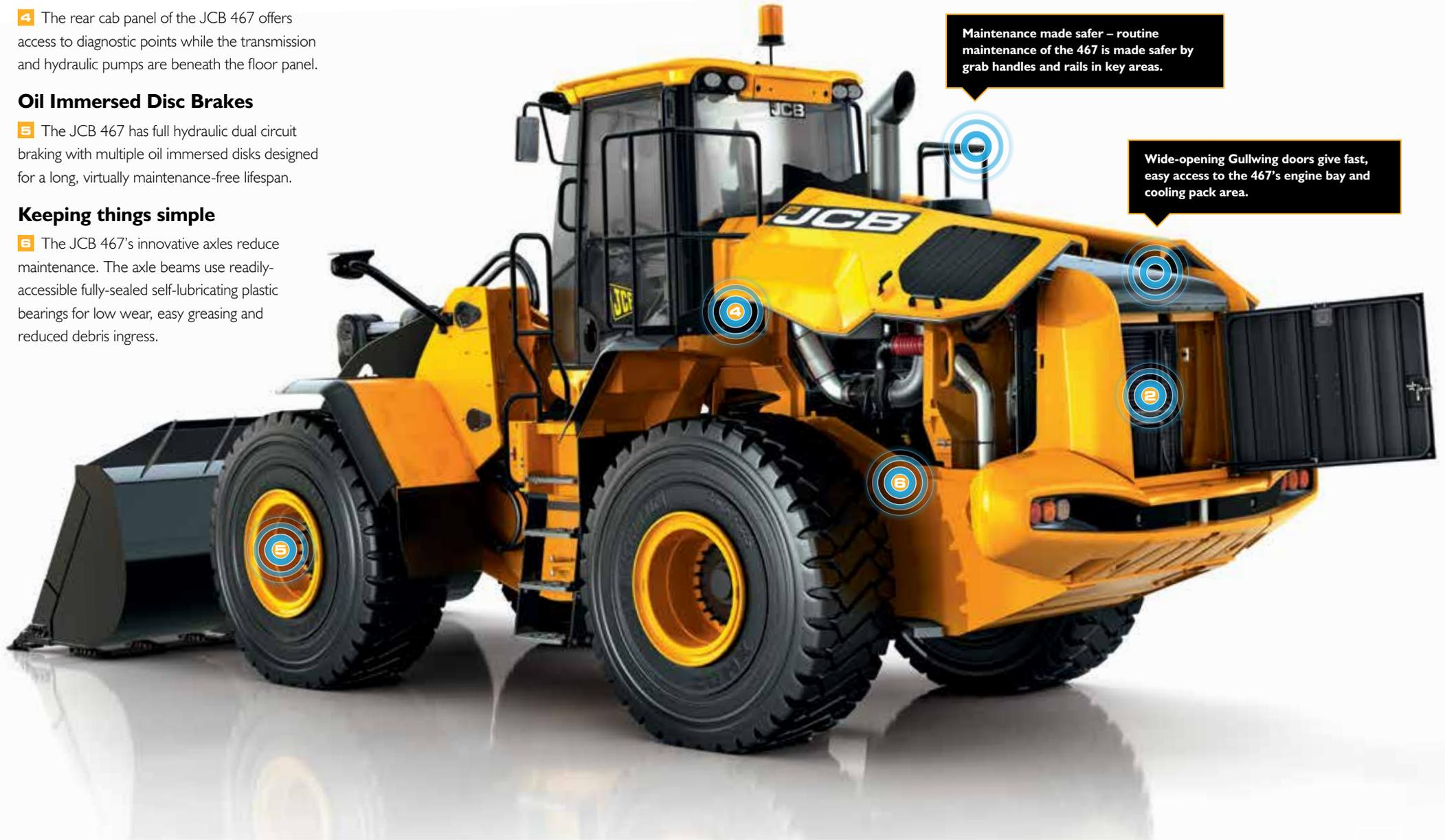
Maintenance made safer – routine maintenance of the 467 is made safer by grab handles and rails in key areas.
