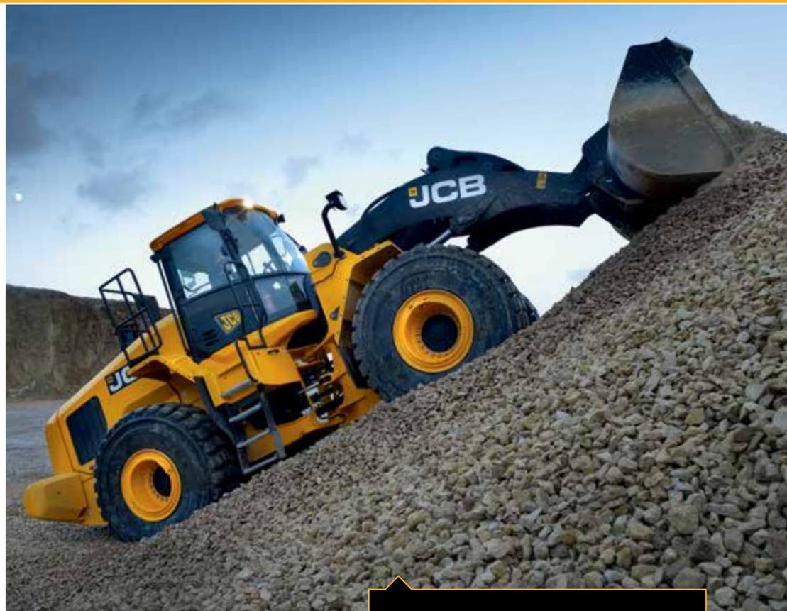
Class-leading climbing and stockpiling capability with high power-to-weight ratio and 27° departure angle. Z-Bar loader design delivers 188kN of breakout force.
